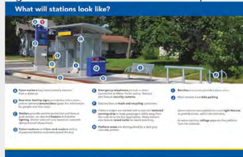
Figure 3.5C.1: Elements of Bus Rapid Transit stop
