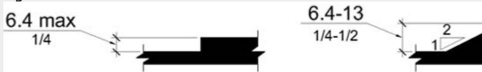
Figure 3.2C.1: Vertical surface discontinuities
