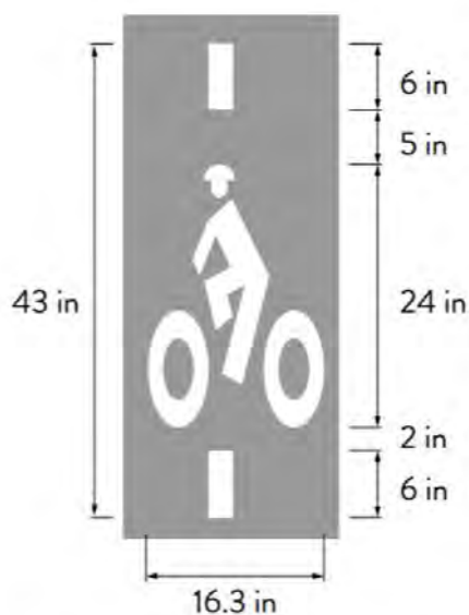
EXHIBIT 4-23: Bicycle Detection Pavement Marking Dimensions
